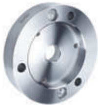
The mounting flange for cylinders with short taper is available in taper sizes 5, 6, 8, and 11. The threaded connection is available in sizes ISO 702-1 (DIN55026, threaded connection), 701-2 (DIN55029, camlock) and 702-3 (studs with nuts). The flanges also fit on the CoAE with center mount.
