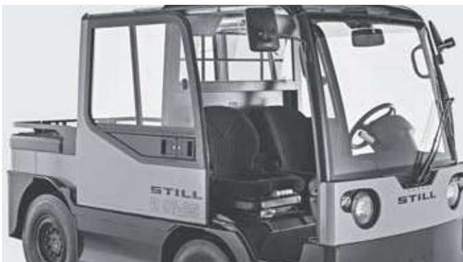
Optional compact sliding door for easy entry and exit even in confined spaces
