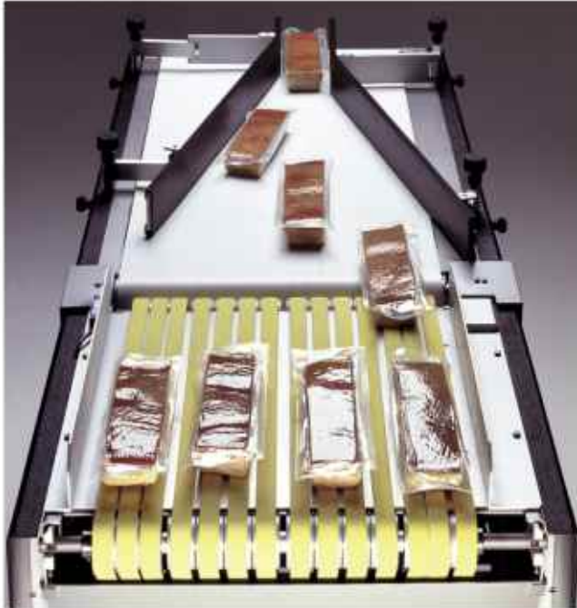
The flexible feed belt control merges up to 6 lines at the same time
