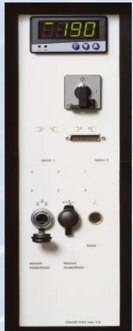
Main switch, test specimen protection and interfaces
