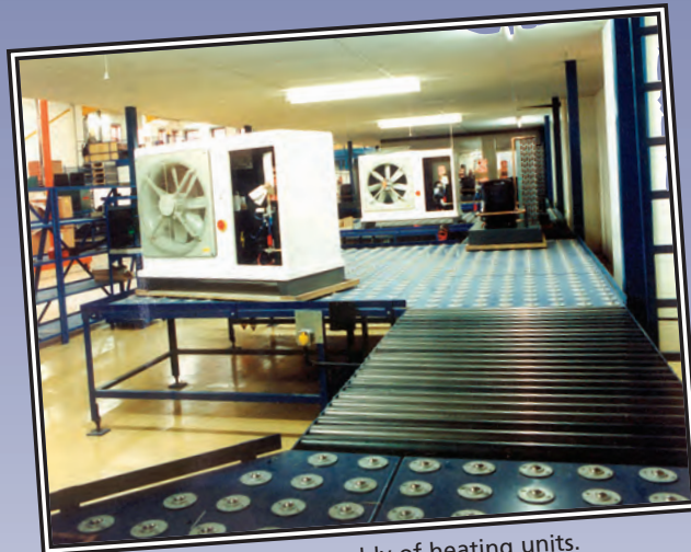
Ball frame for glass handling.
