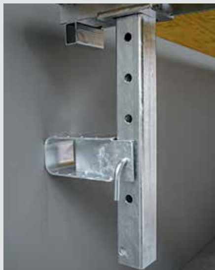
The pressure point of the Support Extension 300 FB is adjustable in 10 cm increments.
