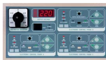
► Three phase equipment synoptic (Independent phase regulation)
