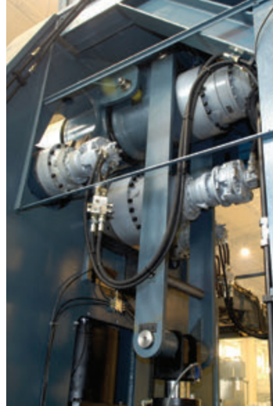
2-4 Drive Top roll Ø 140mm - 430mm
