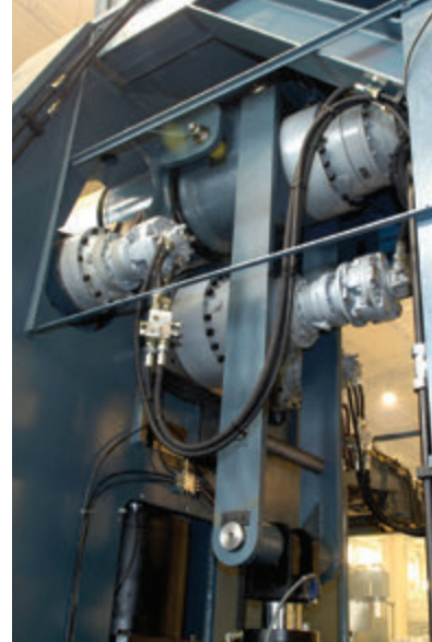
2-4 Drive Top roll Ø 140mm - 430mm
