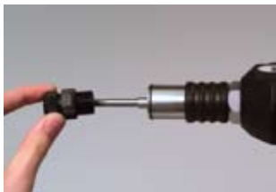
1. Release the nosepiece and contra nut
