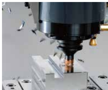
Grooving using standard specs Cutting amount : 150cc/min Material: Carbon steel (for ø16 end mill)
