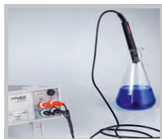
Temperature measurement HZ887 in combination with HM8112-3
