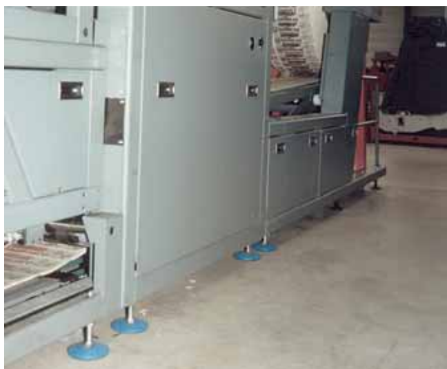
Packaging machine on type N mounts
