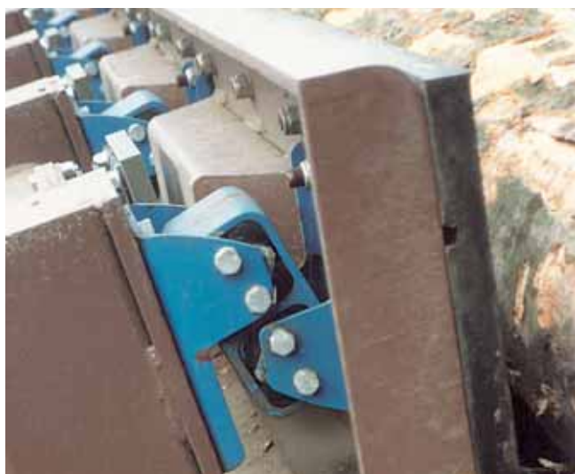
Impact plate equipped with type ESL
