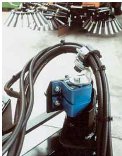
Suspension of a brush in road sweeper
