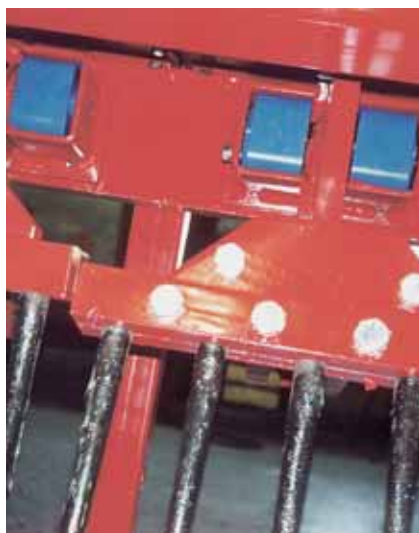
Elastic suspension of a rake in potato harvester
