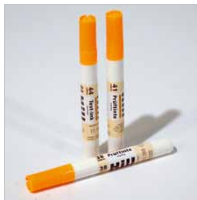
Test inks for surface tension
