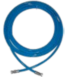
Ref. 18510 Antipulsation hose Ø 3/8" with M16x1,5 fitting, 15m
