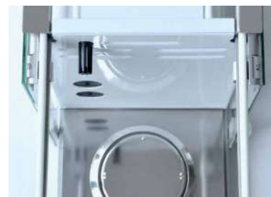
AOS - Ambient observation system records various ambient air conditions what can affect your weighing result. Or shall the balance correct the weighing results with the app BEST?
