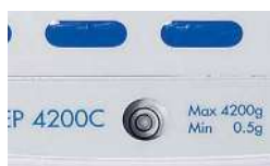
Bubble level located at the front; provides easier adjustment
