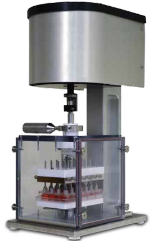
ElectroForce 5500 Test Instrument with 24-Well Plate Fixture
