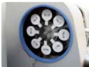
Motorized 8 hollow cathode lamp turret accessory
