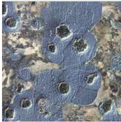
Nodular cast iron etched: DIC
