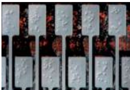
LCD (conductive particles) (episcopic DIC observation)
