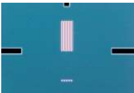
Glass etching pattern (diascopic DIC observation)
