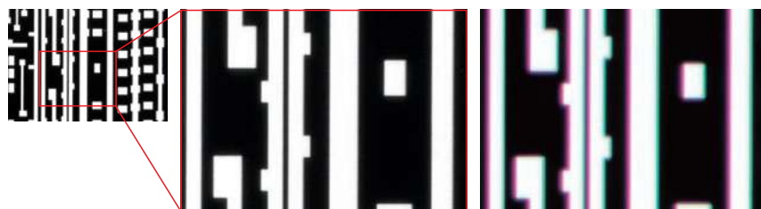
Apochromat optics (captured with SMZ1270+Plan Apo 1x/WF)
