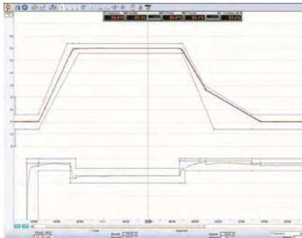
Example of an IEC 60068-2-30 test
