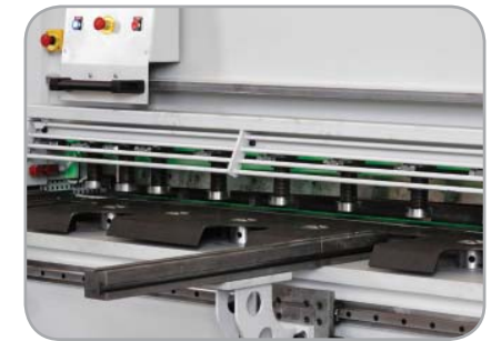
Front guard with 1 swivelling part.
