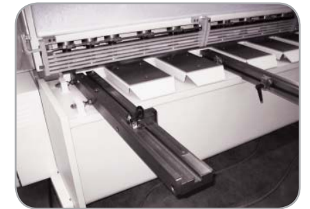
1m Squaring Arm with linear scale
