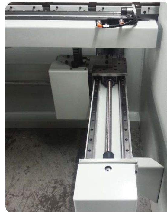
Back gauge with double linear guides on every axis.
