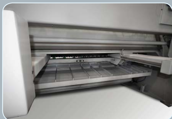
Position 2: Goes down, approximately of 100mm, stops, waiting for the whole length to be cut, not leaving the sheet to bend to the floor.
