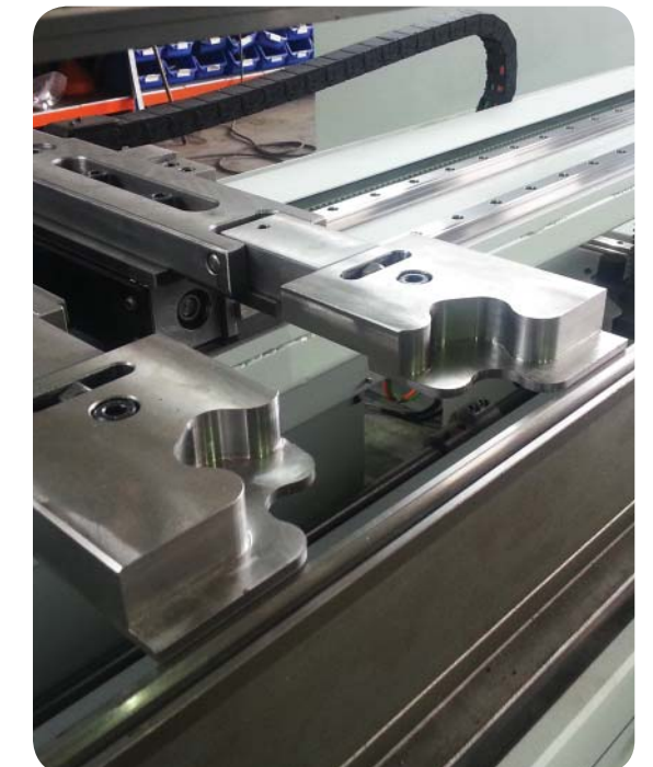
Special Designed Stop Fingers for high Accuracy and maximum Flexibility even for conical bends
