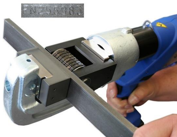
BMH 120 AkkuMarker with a numbering head
