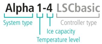
Different ice condenser temperatures are available for each base model, depending on the solvents used:
